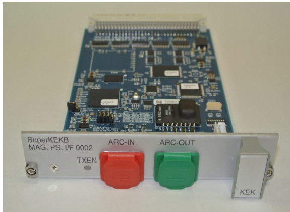
Figure 2: The upgraded PSICM (Power Supply Interface Controller Module), used for the magnet power supply control, for SuperKEKB.
