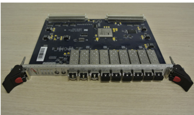
Figure 5: The new Event Generator, VME-EVO.
