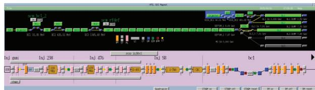
Figure 2: Operation GUI for magnet power supplies.
