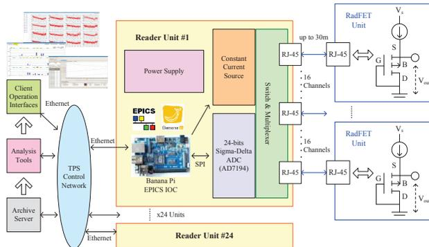
Figure 6: Block diagram of the RadFET readers system.
