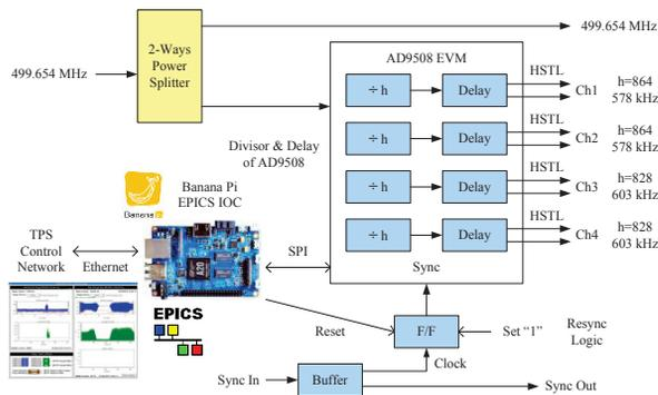
Figure 2: Block diagram of the programmable clock generator.
