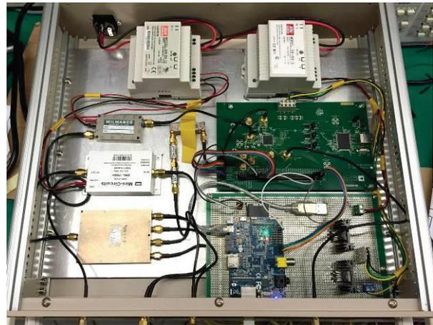
Figure 5: Photo of the prototype DDS signal generator.
