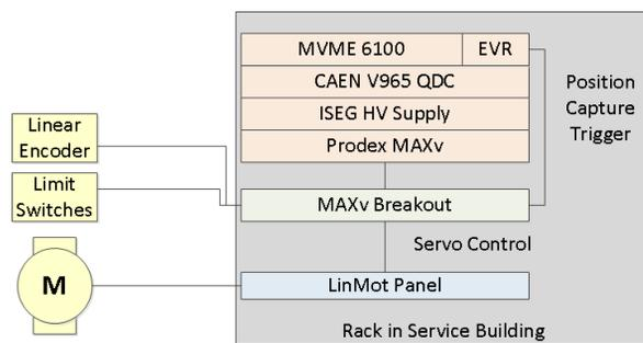
Figure 2: Fast Wire Scanner Control System Architecture.
