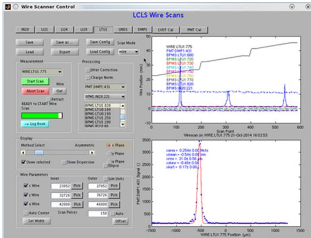
Figure 6: Wire scan graphical user interface showing x, y and u wire scan signals as well as motor position (top right) and individual wire scan profile (bottom right).
