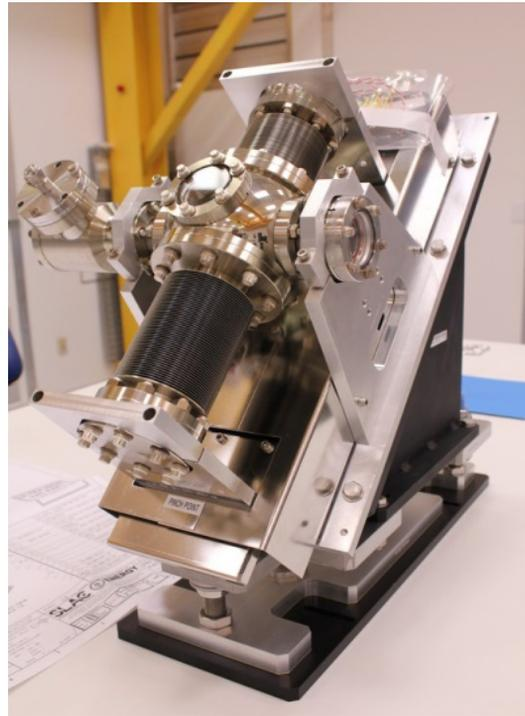
Figure 1: Wire scanner mounted at  $45^\circ$ .
