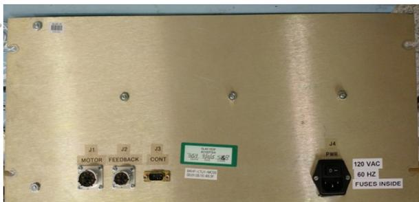
Figure 4: LinMot Panel, Rear View.
