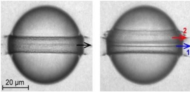
Figure 7: XFEL beams imaged by camera in CXI experimental hutch hitting water droplets. Single bunch beam is seen on the left and two-bunch on the right. The arrows indicate the XFEL beams.
