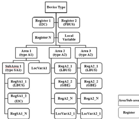
Figure 1: Example of a model of a device.
