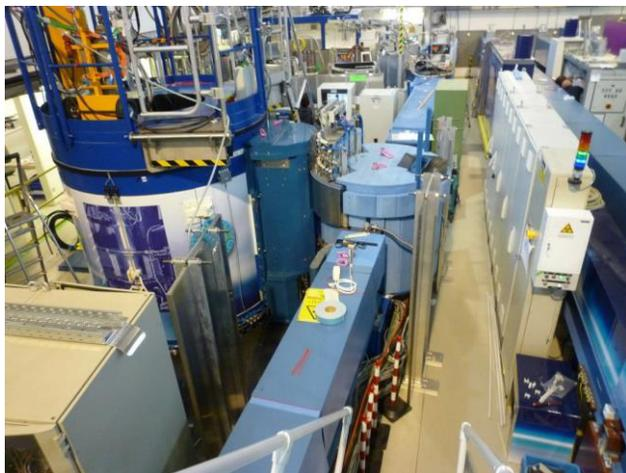
Figure 2: The diffuse neutron scattering instrument DNS.
