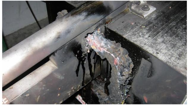
Figure 1: Septa magnet MYR7S03 fire damage.
