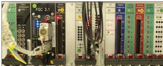
Figure 2: RegFGC3 chassis for the Modulator converter.
