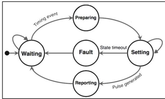
Figure 5: Pulse state machine.
