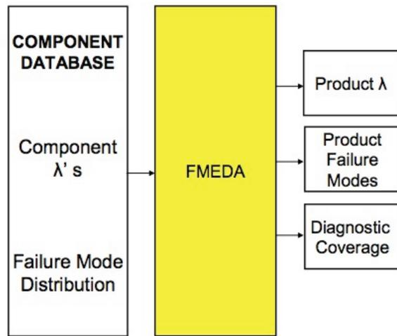
Figure 3: FMEDA inputs and outputs. Source: [6]
