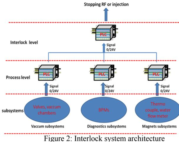
Figure 2: Interlock system architecture
