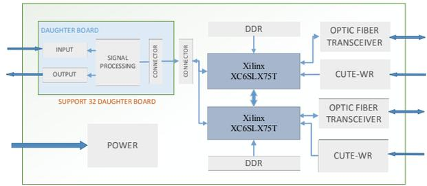
Figure 3: Schematic diagram of the front IO sub-board.
