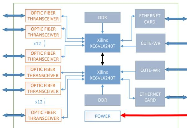
Figure 5: Schematic diagram of the main control board.
