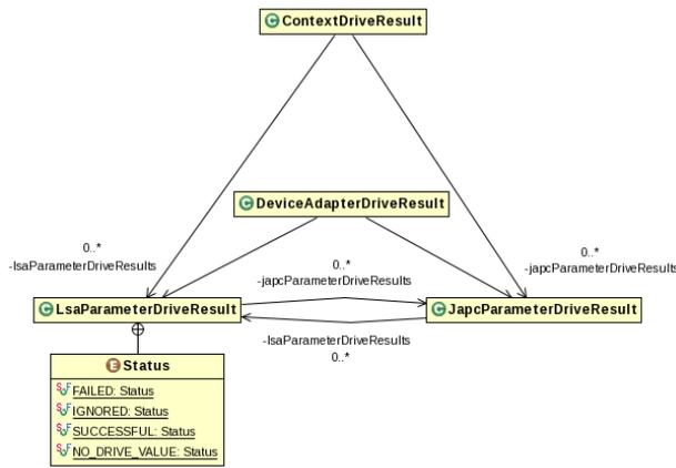
Figure 3: Class diagram showing the refactored LSA data supply results structure.
