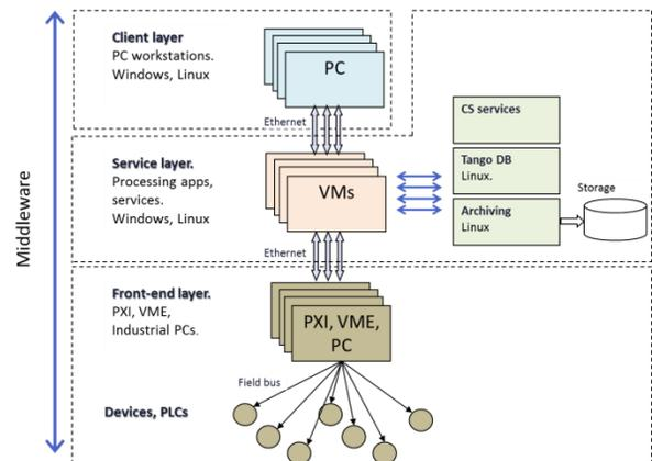
Figure 1: NICA control system layout.
