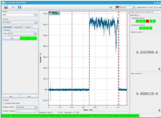
Figure 2: Intensity measurement of a chopped 500  $\mu\text{s}$   $\text{D}^+$  beam pulse with a Faraday-cup.
