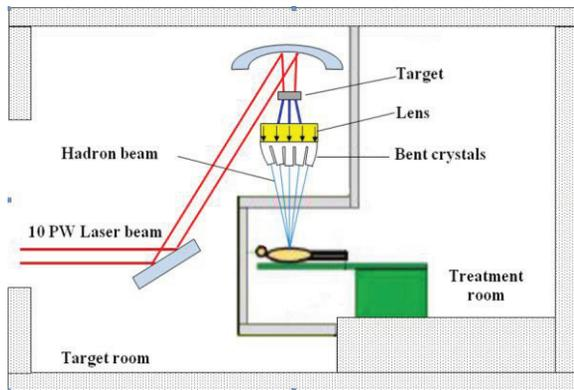
Figure 2: Proposal of an optical-laser gantry system which using mirrors and the phenemem of chaneling in bent crystals as steering, bending and focusing device for hadron beams.
