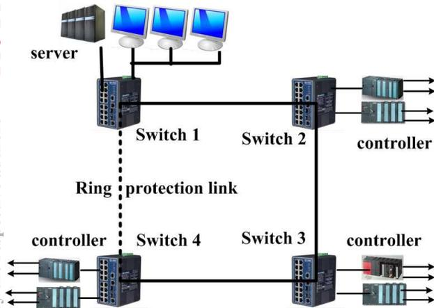
Figure 2: Redundant Ethernet used in the control network for the spallation target. The four switches are equipped with Ethernet ring protection protocol, with which users can establish a redundant Ethernet network with ultra high-speed recovery time.
