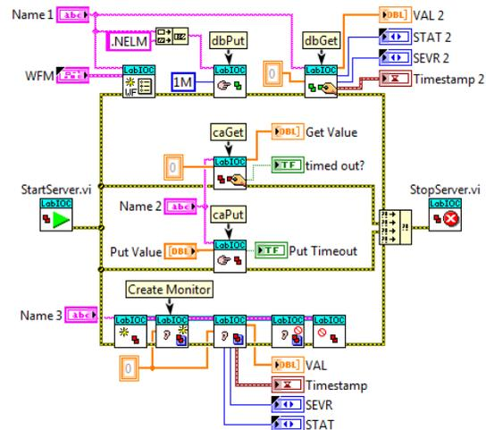
Figure 3: Example of the LabIOC LabVIEW interface.
