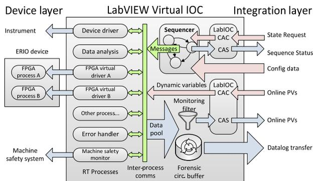
Figure 2: Block diagram of the LabVIEW-based IOC framework.
