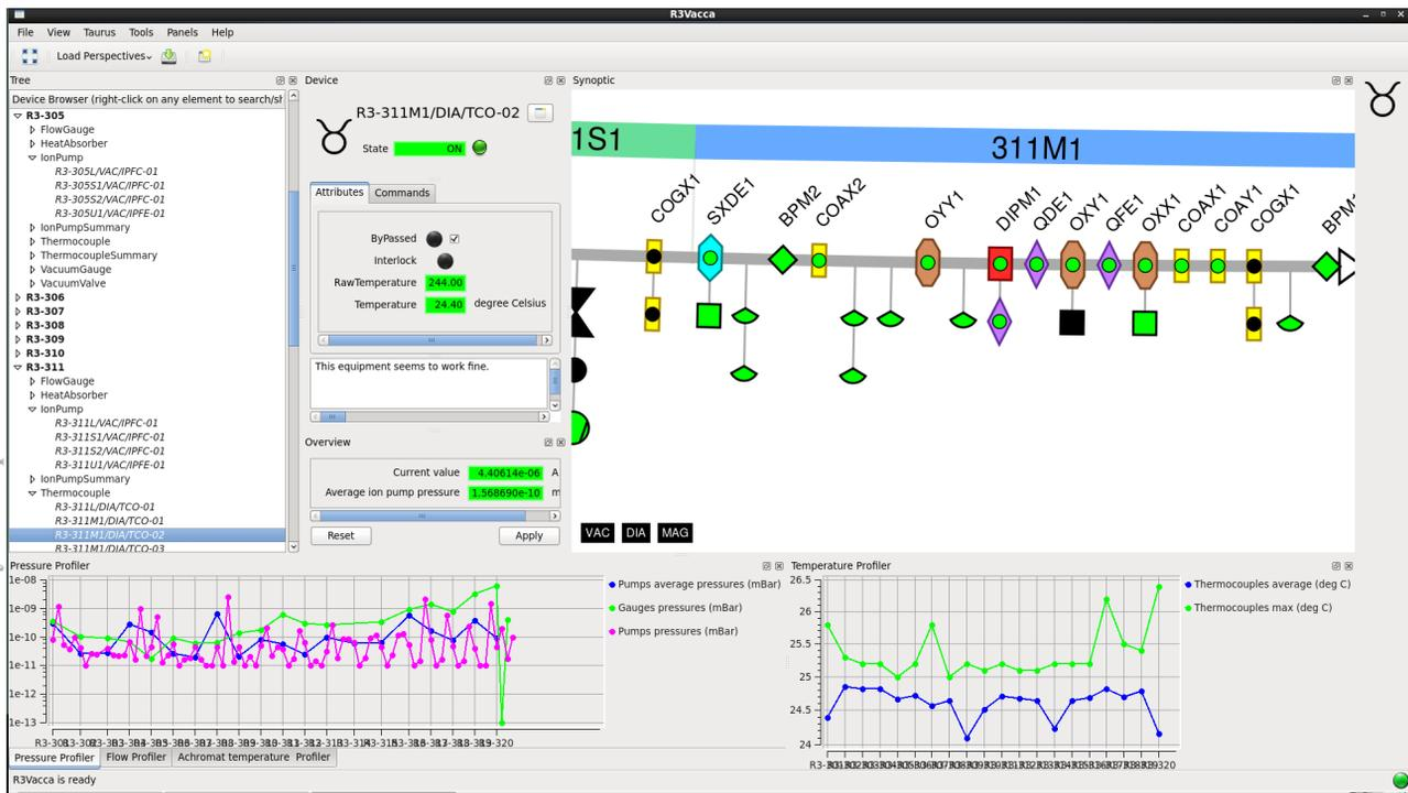
Figure 3: An example of embedding the SVG synoptic widget in a dedicated vacuum monitoring application. The widget responds to user actions such as selecting a device in the tree to the left, by displaying the chosen device, and vice versa.
