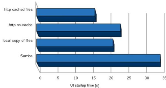
Figure 2: Time to start up the UI for a large SCADA application on a Windows Terminal Server, with Samba and http method.
