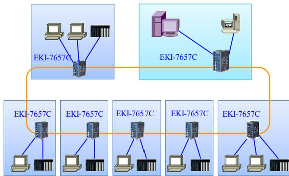
Figure 2: Redundant Gigabit Ethernet used for injector II.
