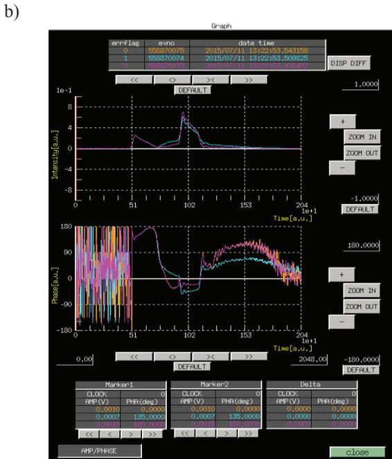
Figure 4: Management GUI for abnormal WFM-DAQ system. a) List panel of abnormal signal. b) GUI of an abnormal waveform viewer.
