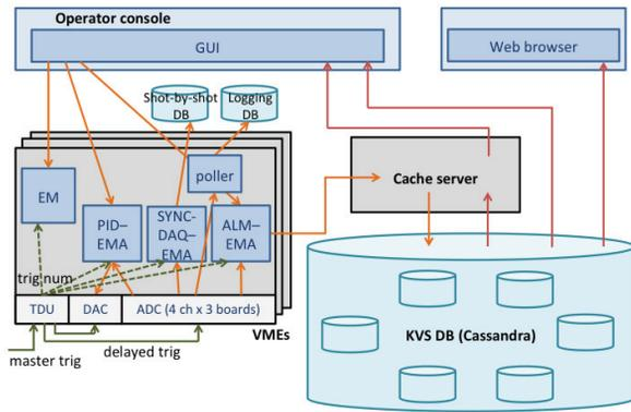
Figure 2: Diagram of abnormal waveform DAQ system.
