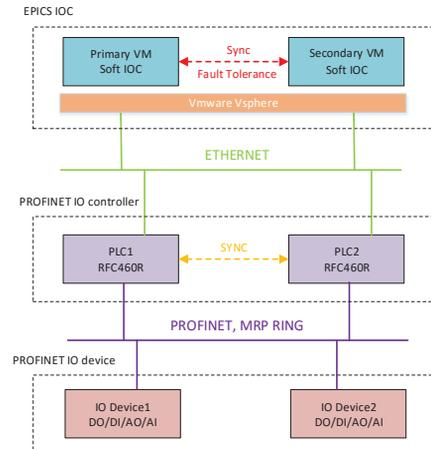
Figure 1: System architecture of the redundant control system.
