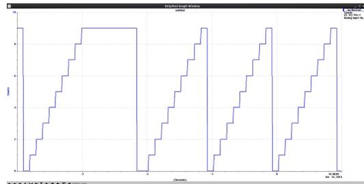
Figure 3: Switch-over of the softIOC monitored by Striptool.
