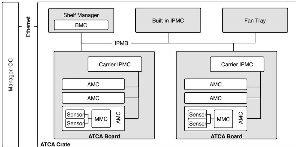
Figure 1: Typical IPMI system in an ATCA crate.
