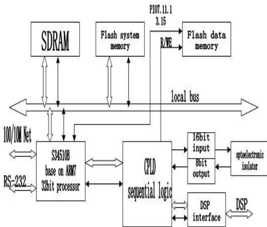
Figure 3: The structure of the ARM controller.
