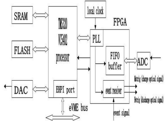
Figure 4: The structure of the DSP processor.
