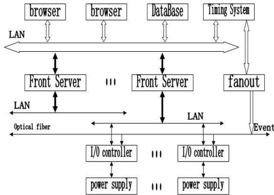
Figure 2: The structure of the power control system.
