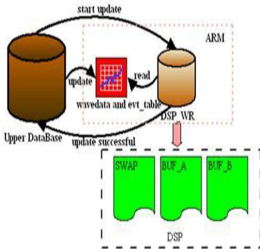
Figure 6: The waveform data download flow chart.
