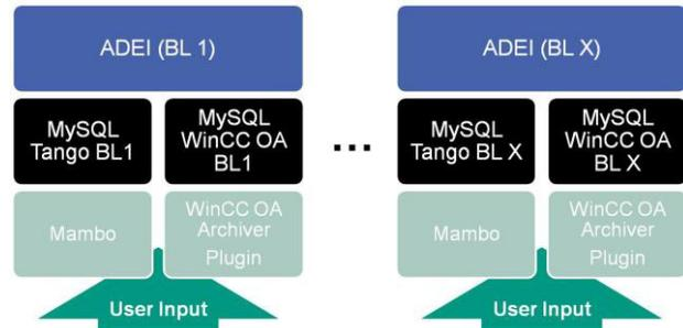
Figure 4: The different software layers of the ANKA Archiving system. The user configures the logged data, which is afterwards saved in a MySQL database and finally presented by ADEI.
