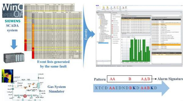
Figure 3: Analysis flow of the gas system alarms.
