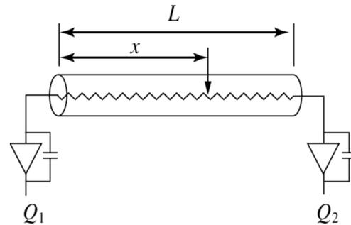
Figure 2: Principle of a charge-division neutron detector.
