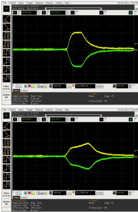
Figure 3: Examples of differential pulse-shapes from <sup>3</sup>He tube.
