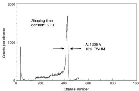
Figure 1: Pulse-height spectrum from  $^3\text{He}$  tube.
