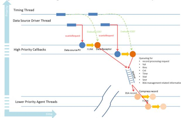
Figure 6: Consideration for parallel callbacks for multi-core system
