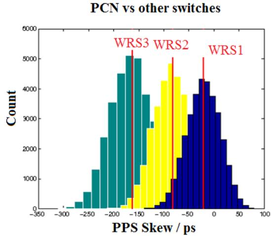
Figure 3: PPS skew between PCN and other switches
