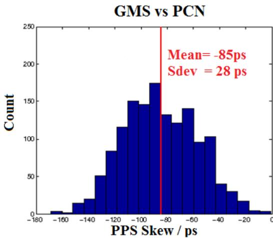
Figure 2: PPS skew between PCN and GMS
