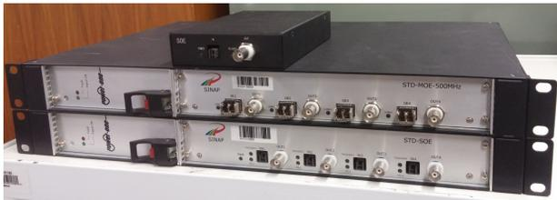
Figure 1: Optical to electrical converters STD-MOE, STD-SOE and SOE.
