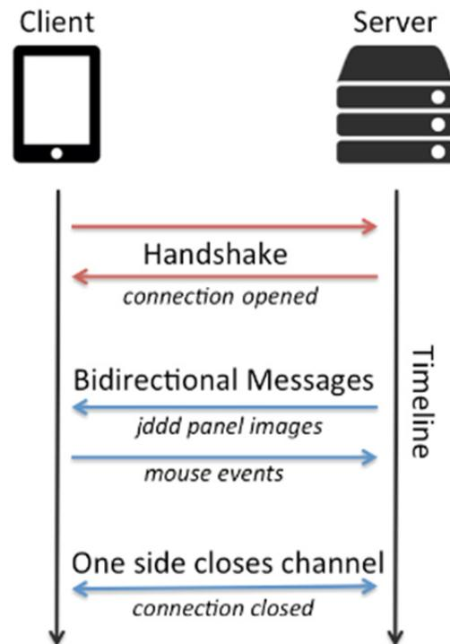
Figure 1: Using WebSockets for client / server communication.
