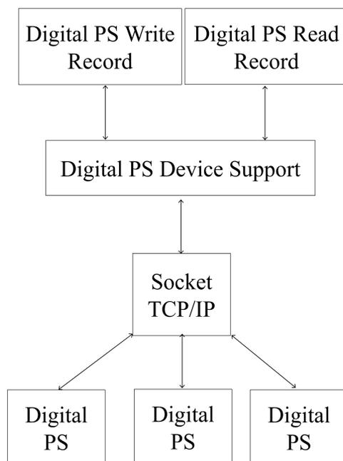
The bottom of the structure is digital PS. Above the PS is Ethernet interface and use TCP/IP as low level transfer protocol. In the middle layer is device support of EPICS architecture. The device support has two functions. First function is a periodic that sends a read command string to PS in every one second and receives current state of the PS. The second function is sends a write command string to PS. The top of the structure is record support.
