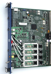
FIG. 8: Photograph of prototype of BPM readout board (double width VME card).
