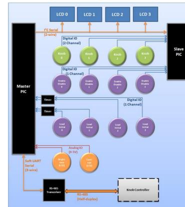
The knob box has two main tasks, each executed by a PIC16F1937 microcontroller
