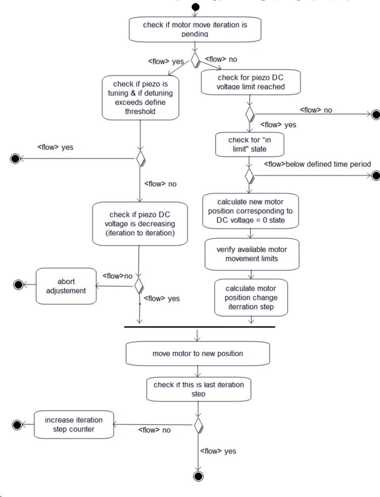
Figure 4: Piezo dynamical range optimization algorithm overview
