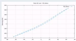
Figure 1: Piezo tuning range characterization
