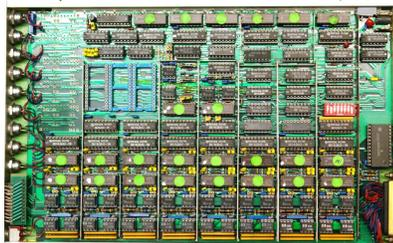
figure 1: CAMAC MPS module.
