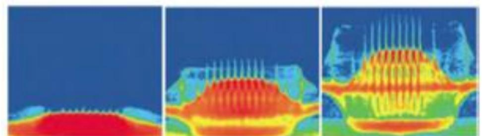
Using the LANSCE proton beam allows for multiple images taken at a wide range of intervals, capturing a movie of the event where the frames may be spaced from one second to 10<sup>-7</sup> seconds apart.
