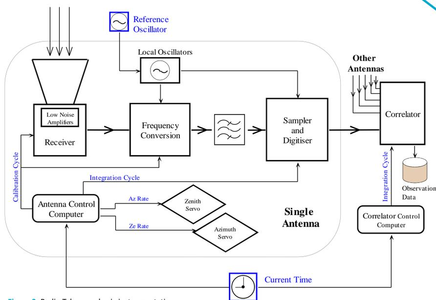
Figure 2: Radio Telescope basic instrumentation
