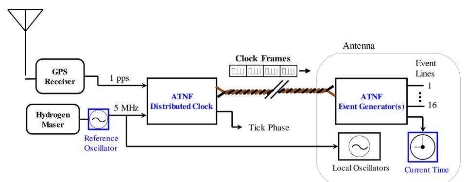
Figure 3: Basic architecture of the timing system
