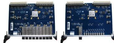
Fig. 5: The EVG (event generator) and EVR (event receiver) in timing system, which is provided by Shanghai institute of applied physics, Chinese Academy of Sciences.
