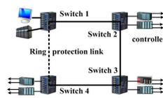
Fig. 2 Ethernet ring protection
