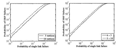
Fig. 4 Left: Reliability for the topologies in Fig. 3(a) and (c) are compared. 5 or 10 means the number of switches in a ring.
